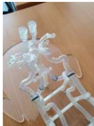
Figure 2: Detail view of the arterial network of the prototype.
