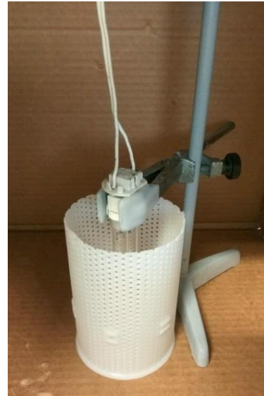
Figure 3. UV disinfection of plastic tanks used in the manufacture of cheeses.
