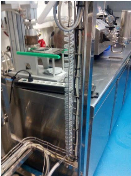
Figure 1. UV-C device used to deactivate microorganisms in opaque liquid foods.
