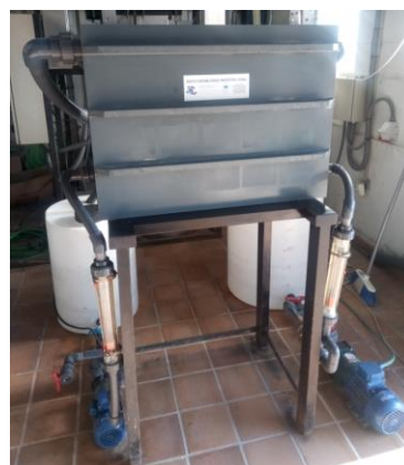
Image 2: front view of the pilot plant scale prototype in the parallel flat electrode configuration, with a treatment capacity of 15 kg.
