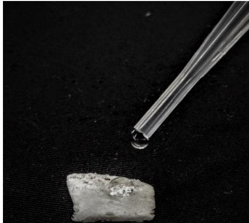
Figure 1. Aerogel showing its hydrophobic capacity.
