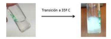
Image 1: Gelificaction process at 35°C
