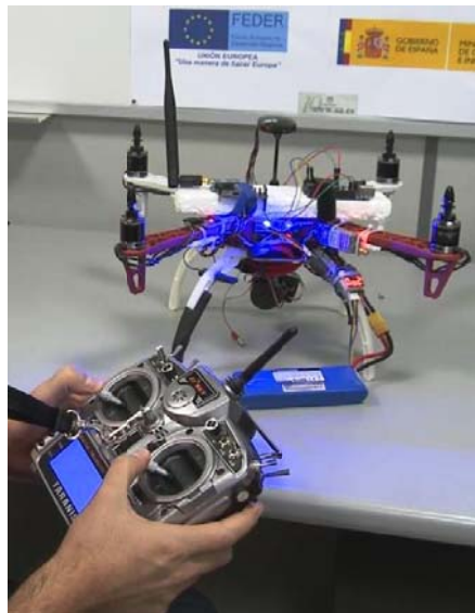
Image 2: UAV control system
