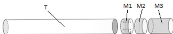
Image 1: tobacco column (T) and combined filter by: the primary membrane (M1), the intermediate membrane (M2) and the outer membrane (M3).
