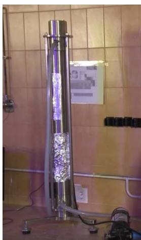
Image 1: UV light emission disinfection device
