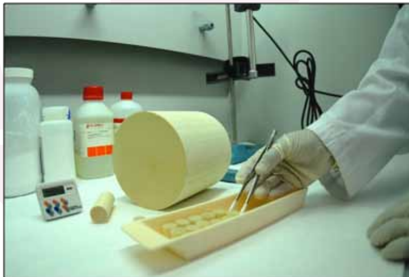
Monolithes used for supporting the catalytic trap to be installed in engines.
