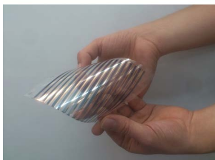
Image 2: Flexibility of the thermoelectric device
